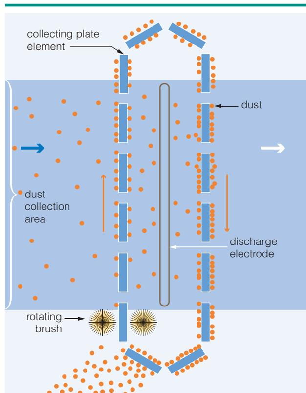
**Figure 7 MEEP schematic** (Hitachi, 2012)
