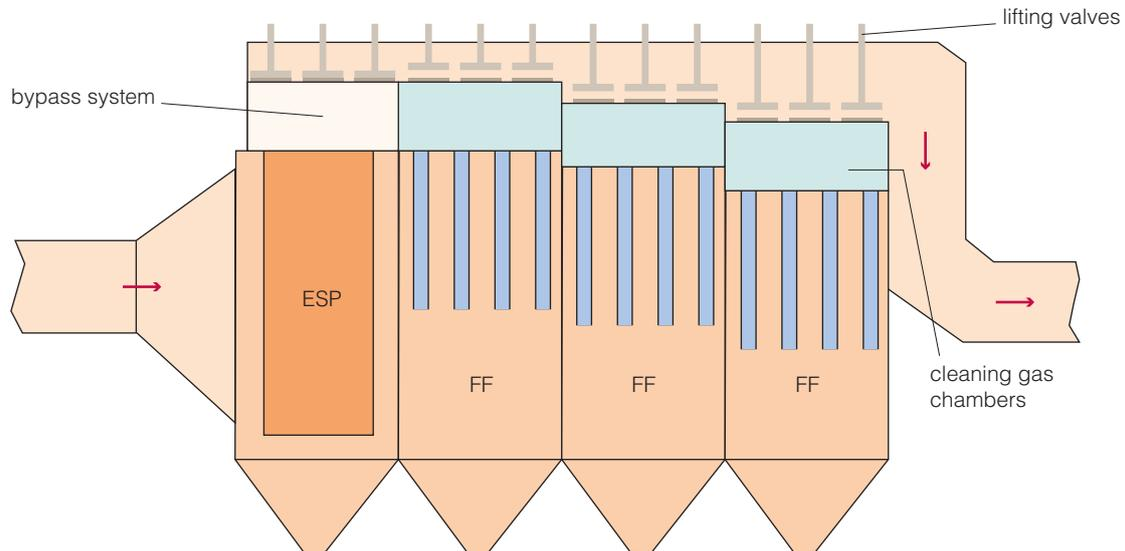
**Figure 20** EFIC schematic (Zheng and others, 2011)
