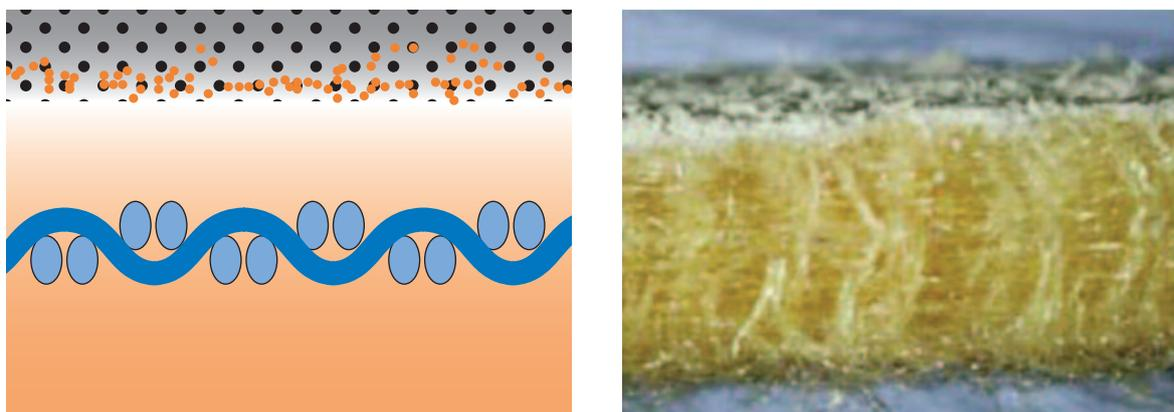
**Figure 13 Needle felt filter schematic** (Popovici, 2011)
