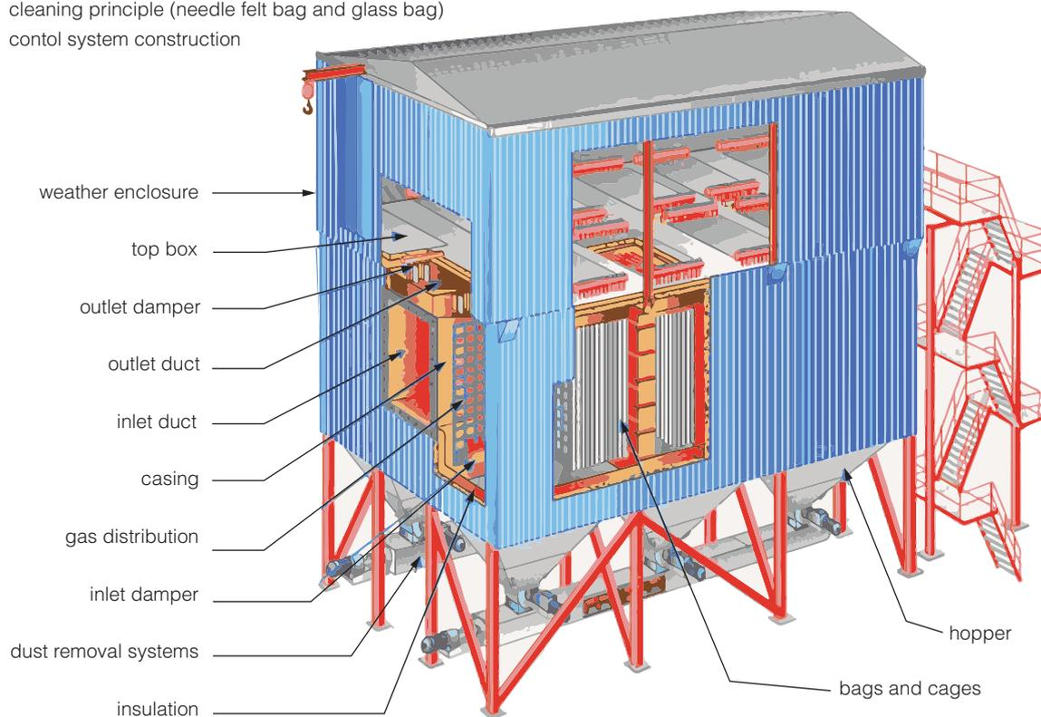
**Figure 11 PJFF schematic** (FLSmith, 2012b)
