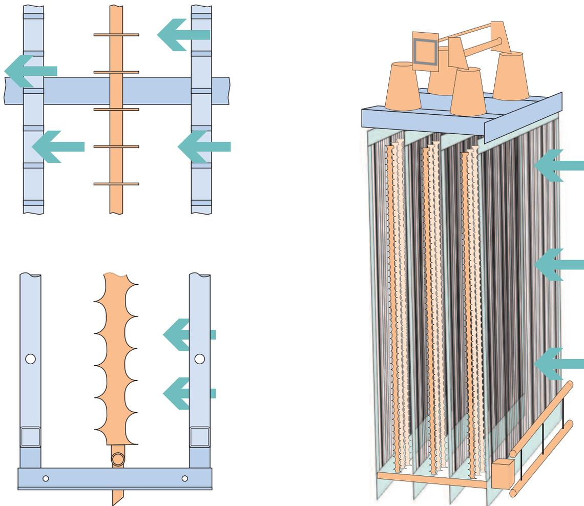
**Figure 9 Cross flow ESP schematic** (Back and Francis, 2006)
