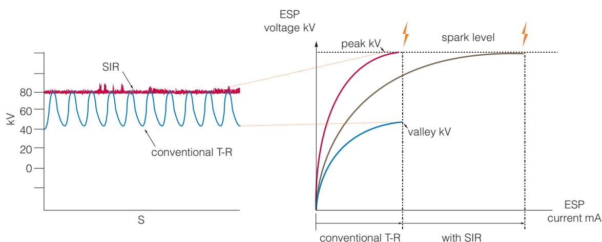
**Figure 4** Ripple difference between SIR and conventional T-R (Ranstad and other, 2011)
