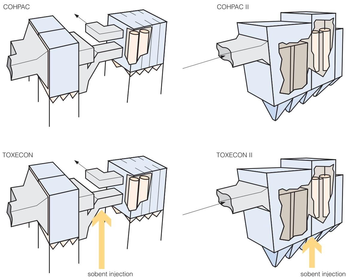
**Figure 17 Schematics of COHPAC, COHPAC II, TOXECON and TOXECON II (Zhu, 2003)**
