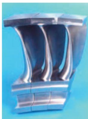
The drum-type HP/IP blade construction features an integrally shrouded blade design concept. The integral shrouds provide two basic functions: first, they form a circumferential steam path boundary allowing efficient seal designs to be utilised; and second, they provide individual blade tip support between neighbouring blades in each blade row.
