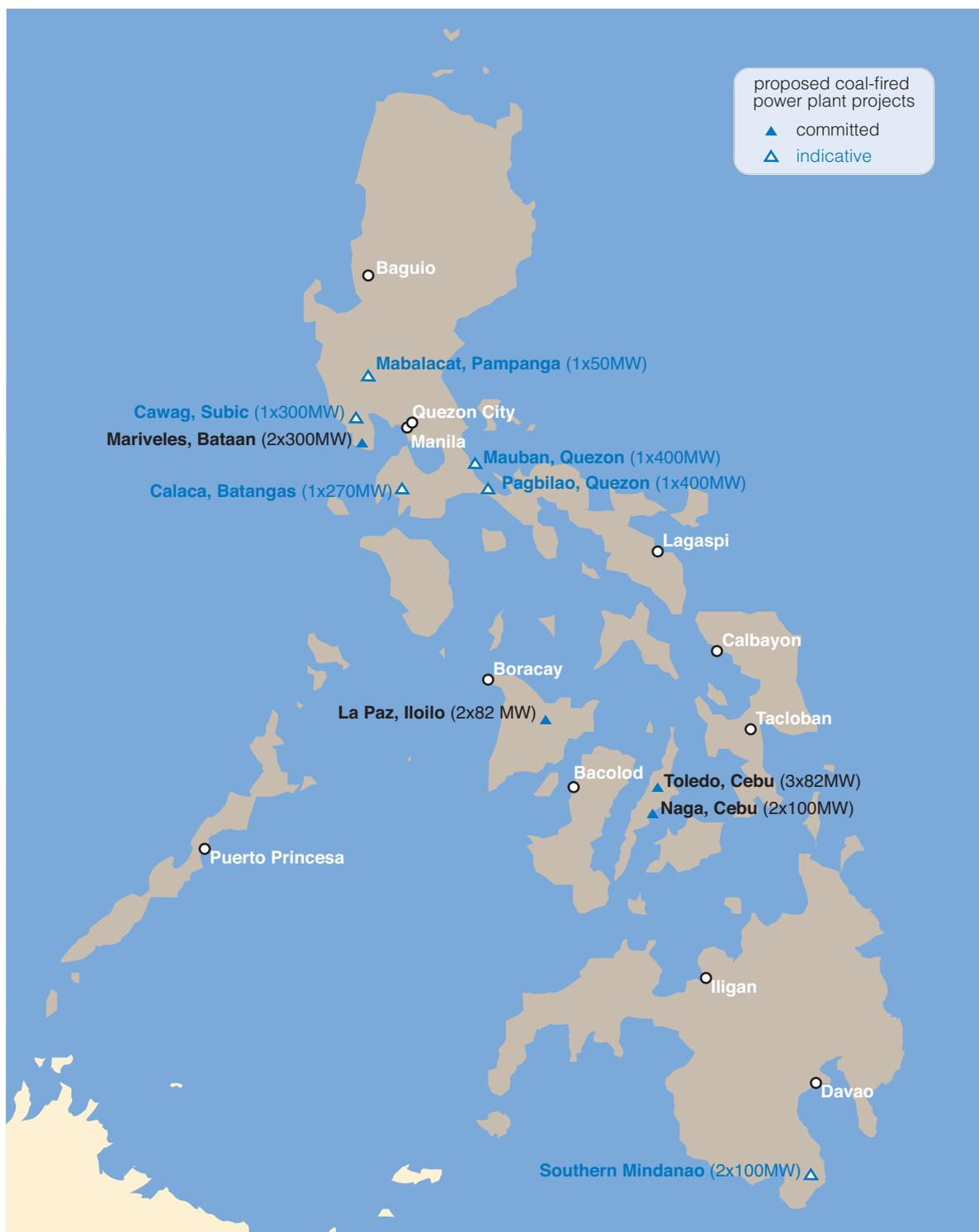
**Figure 5 Proposed new coal-fired power plants in the Philippines**
