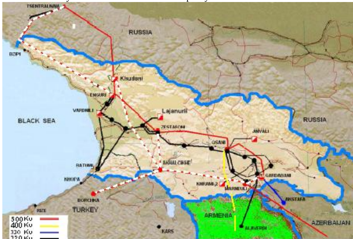
Figure 2.4 – Georgia – Network reinforcements
