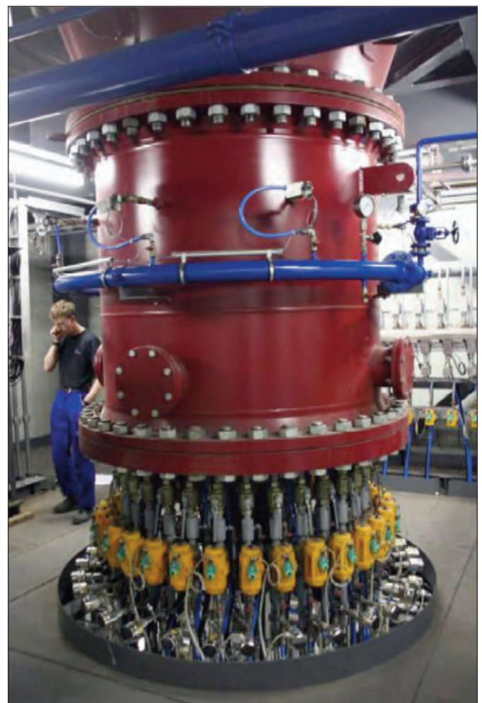
Figure 9 Pressure hopper with distributors (32 in total) (Buegler, 2009b)
