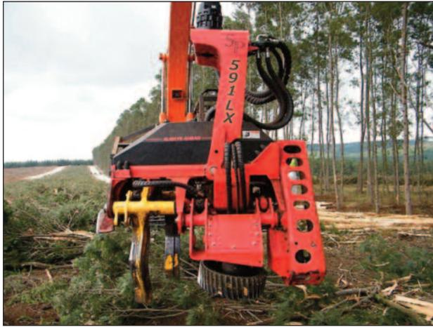
**Figure 8 Tree harvester** (photograph courtesy of Logging On Newsletter)
