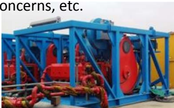
6000HP AC Fracturing pump
