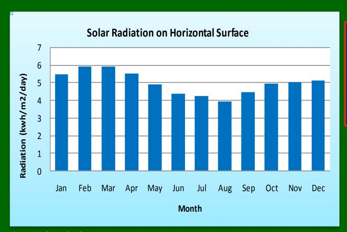
Monthly solar radiation on horizontal surface is about 4 to 6 kWh/m²/day
